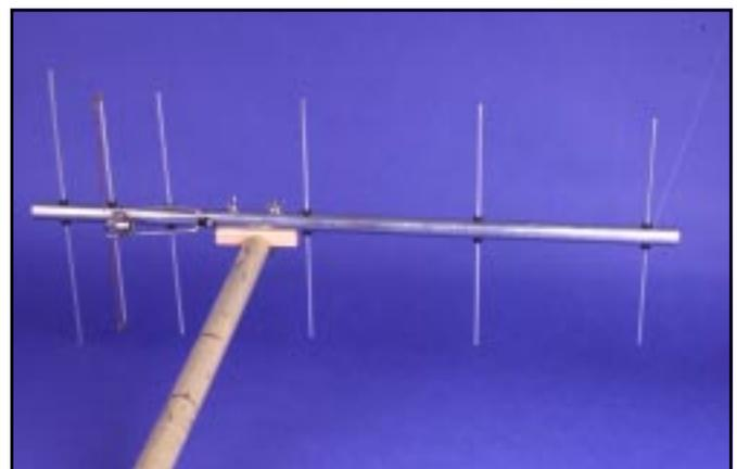
**Fig 7—70-cm Yagi mounted to a 1/4-inch boom.**
